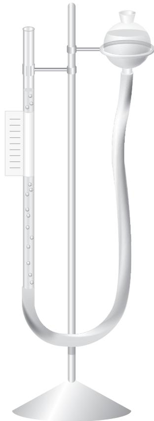
the burette and add BROMOFORM thru the bulb until it is up to the 25 ml. mark.
